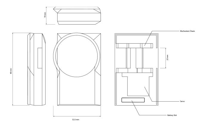
Here we can see the various components needed to be housed within the case that we designed and 3D-printed. The apparent thickness of the case is around 9mm, while the true thickness is 19. The most difficult piece to fit into the case was the servo motor, so ideally for future iterations, we might seek a smaller servo or motor to replace the current one we used.
