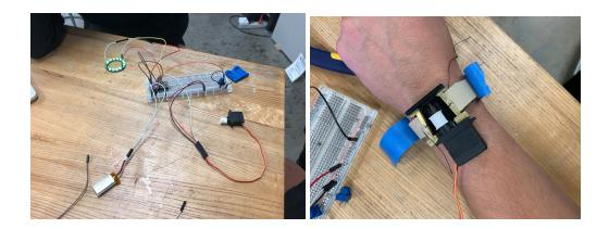
Once the basic electronics were functional, we did a fair amount of tuning in the code to ensure that the rate and extent of motion were both comfortable and actually mimicked the timing of a breathing pattern. In addition, the colors and brightness of the LEDs needed to be tuned. We wanted to ensure the brightness was controlled so it would not strain the user's eyes with continuous usage. We also
