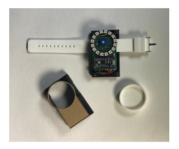
5. Secure the case lid onto the bottom. Place the dial onto the potentiometer. Your Calm.io is now complete!
